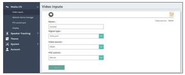
If the desired video source is network camera, a login authentication with the camera is required firstly in the [ Network device manager ] setup tab of [ Media I/O ].
